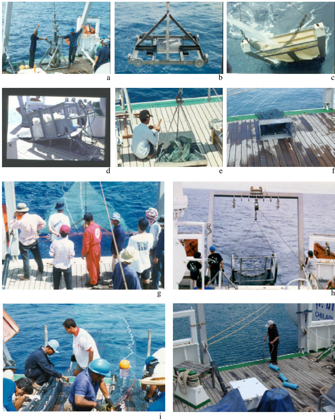
Figure 2 Sampling gear: a. Olsen box corer (BC); b. Smith-McIntyre grab (G); c. Ockelmann sledge (OS); d. Pierce-Rothlisberg hyperbenthic sledge (HS); e. triangular dredge (TD); f. rectangular dredge (RD); g. beam trawl (BT); h. Agassiz trawl (AT); i. otter trawl (T); j. baited trap (Trap).
